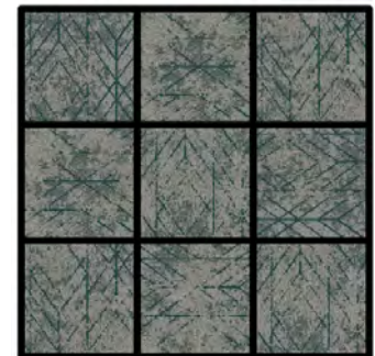
24" X 24" RANDOM CUT TILE QUARTER TURN INSTALLATION
