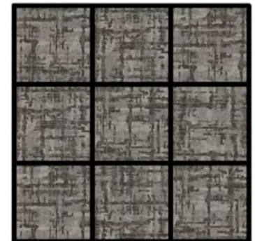
24" X 24" RANDOM CUT TILE QUARTER TURN INSTALLATION
