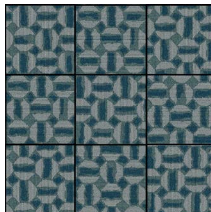
24" X 24" RANDOM CUT TILE QUARTER TURN INSTALLATION
